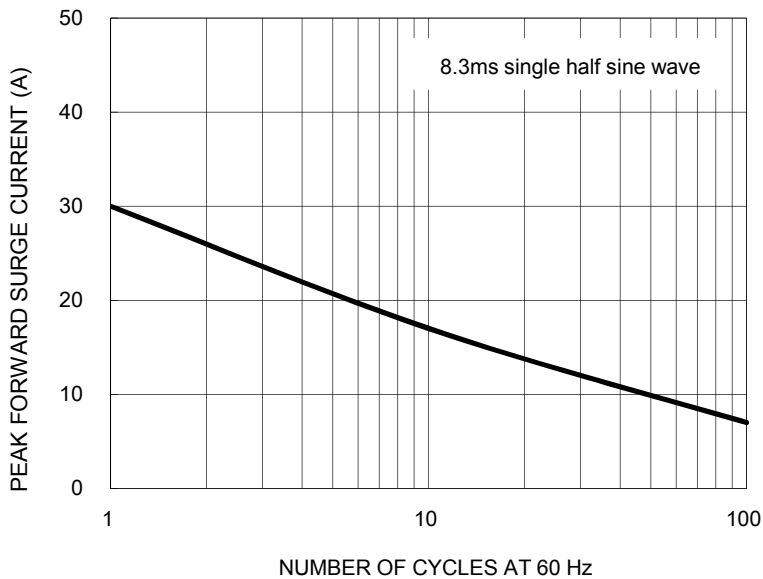
FIG. 3 MAXIMUM NON-REPETITIVE FORWARD SURGE CURRENT
